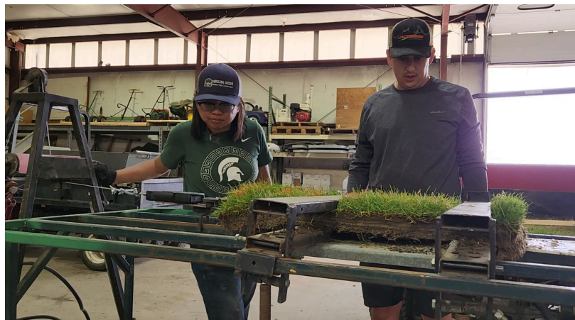
Figure 2. Measurement of sod harvestability (tensile strength) at Hancock Turfgrass Research Center, East Lansing, MI – 2023: (1) a Calrochan Sod Puller was used to pull apart a 1 ft × 1.5 ft sod piece, and (2) a digital force gauge was used to measure the force required (lbs · force) to pull sod apart.
