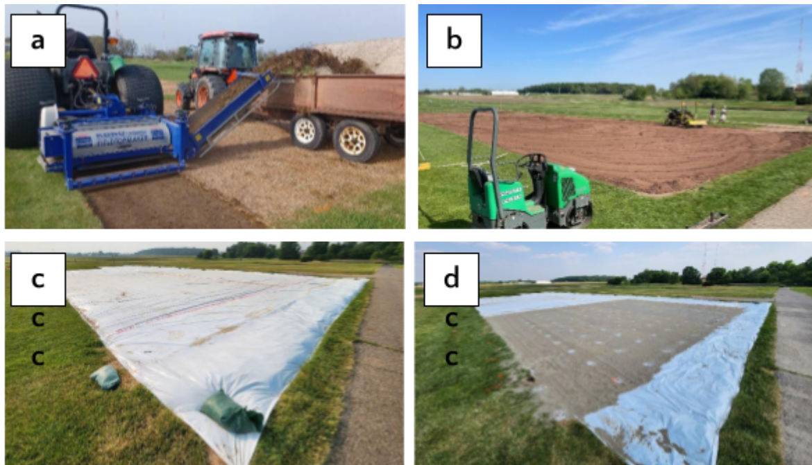
Figure 1. Sod grown on plastic establishment at Hancock Turfgrass Research Center, East Lansing, MI in June 2023. (a) DuraEgde was used as a base for sod grown on plastic establishment. The area was laser-graded to have a 1% slope. (b) A white plastic was laid down on the area. (c) Sand (1-inch depth) was topdressed on top of the plastic sheet.
