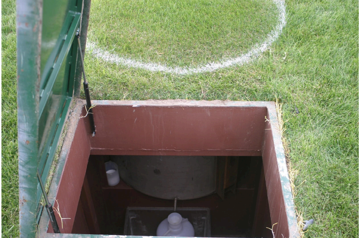
Photo: Lysimeters used for measuring nutrient leaching at the Hancock Turfgrass Research Center.
